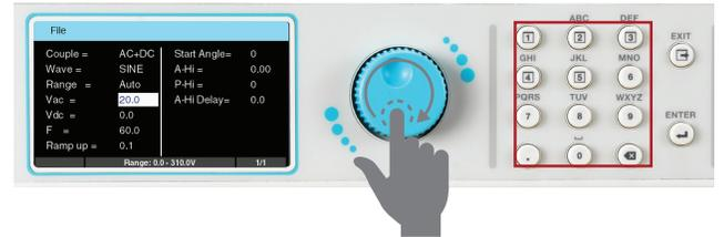
11. Use the rotary knob or keypad to edit the test parameter value. The available range or settings for the test parameter being edited will be displayed at the bottom of the screen. Once the desired value of the test parameter is entered press the rotary knob or the ENTER key on the keypad to save the value and move to the next test parameter:
