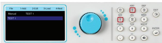
6. To start adding a test file press the number 1 key on the keypad to select Add:
