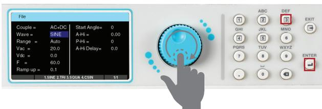
6. To edit the test parameters use a combination of the rotary knob and keypad, as explained in the previous sections. Once all the test parameters have been edited, press the EXIT key on the keypad to view the list of test files and press the EXIT key again to go back to the test menu.
