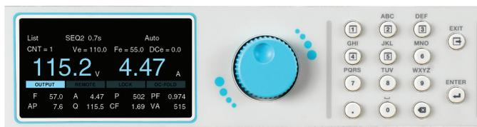
2. The user can press the OUTPUT/RESET key at any time during the test to end/abort the test.
