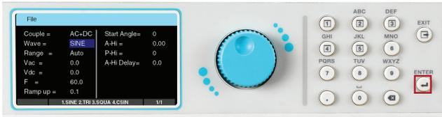
10. The test parameters can be edited in the exact same manner as the system parameters, using a combination of the rotary knob and keypad. To edit a test parameter use the rotary knob to highlight the parameter and press the rotary knob to edit the parameter:
