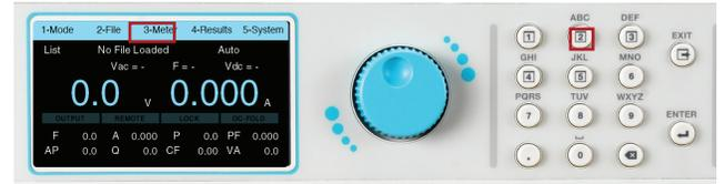
3. The File screen will be displayed and the selections on the menu bar will change. If there are no previously saved test files for List Mode the screen of the File menu will display the selections to Add, Edit or Load a test file on the menu bar. The Next selection on the menu bar will not do anything:
