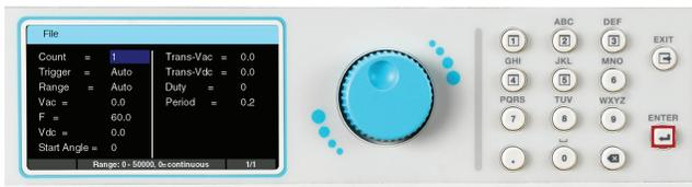
8. The test parameters can be edited in the exact same manner as the system parameters using a combination of the rotary knob and keypad.
