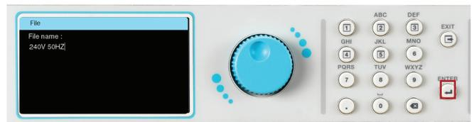
7. The next screen will display all the test parameters for the copied file. Use a combination of rotary knob and keypad if you wish to edit the test parameters. Press the EXIT key and the screen will display the newly copied test file along with other files:
