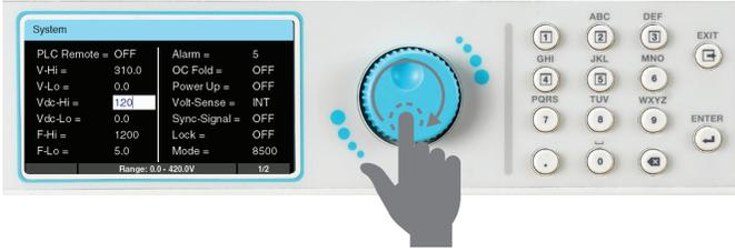
6. Press the rotary knob or the ENTER key on the keypad to save the value. The parameter will be saved and the next parameter will be highlighted.
