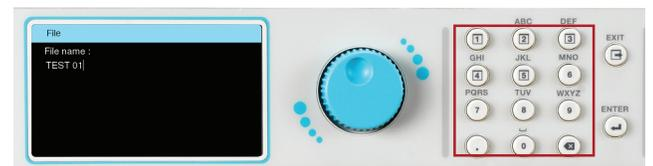
7. After entering the file name press the ENTER key on the keypad to save the file name and display the Program Setup along with the first sequence. The next screen will also display the Add and Edit option on the menu bar:
