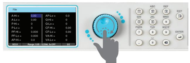
The Program Setup and sequence parameters can be edited in the exact same manner as described in the previous sections, using a combination of rotary knob and keypad.
