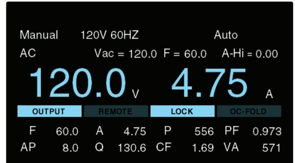
**OC – FOLD** – If the OC-FOLD parameter is enabled and test is performed OC-FOLD will be highlighted on the screen.
