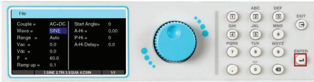
10. The test parameters can be edited in the exact same manner as the system parameters, using a combination of the rotary knob and keypad. To edit a test parameter use the rotary knob to highlight the parameter and press the rotary knob to edit the parameter:
