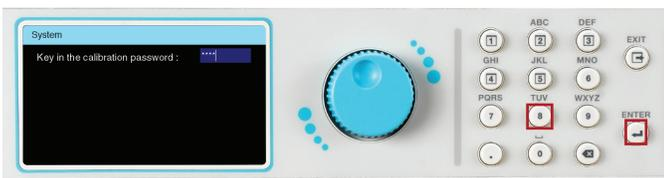
Calibration main screen will appear. The output and remote sense terminal (L to Ls and N to Ns on the rear panel output terminal lug) must be shorted during the calibration.
