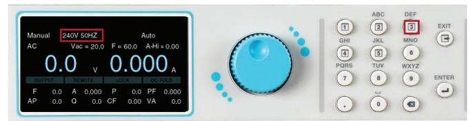
4. The power source will start outputting if you press the OUTPUT/RESET key on the front panel. Make sure all of the output connections are secure and all other safety precautions are taken.
