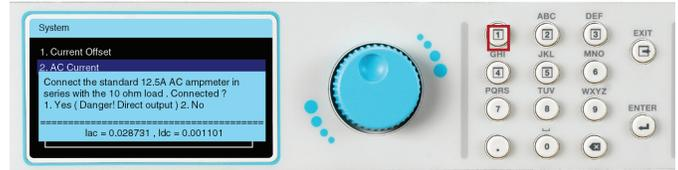
Observe the RMS reading of AC current meter.
