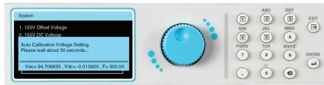
Wait a moment, the frequency setting will automatically change from 50Hz to 1200Hz. (This step does not require any action. This item is the calibration of the AC set value in the frequency range of 50Hz~1200Hz.)
