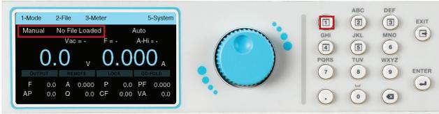
2. Once the Mode has been set to Manual press any key to drop down the menu bar then press the number 2 key on the keypad to enter the File menu:
