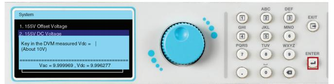
Input the Vdc measurement of the DVM.
