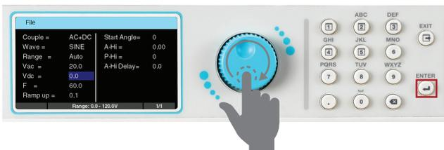
12. Once all test parameters have been programmed press the EXIT key on the keypad and the screen will display your newly created test file (along with other test files that may have already been saved):
