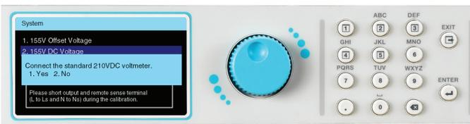
Input the Vdc measurement of the DVM. Press the ENTER key to view the next page.
