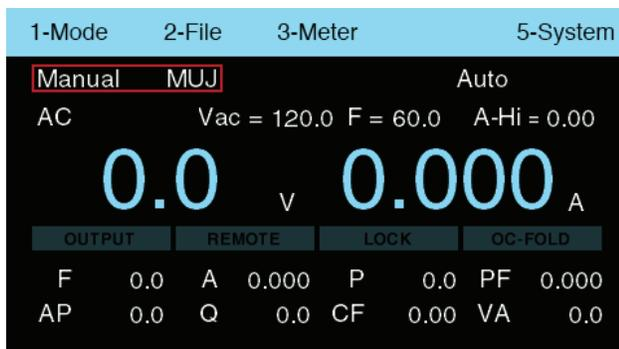
The drop-down menu will display Mode, File, Meter, and System. The output mode and test file name will also be displayed on this screen (marked in the red box) on the image above. Each selection on the menu bar is associated with a number. Use the numeric keypad and press the number for the menu that you would like to enter.
