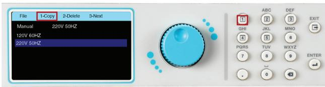
4. The following message will appear on the screen to confirm if you would like to proceed with copying the selected file. Press the number 1 key on the keypad to select Yes, or press the number 2 key on the keypad to select No:
