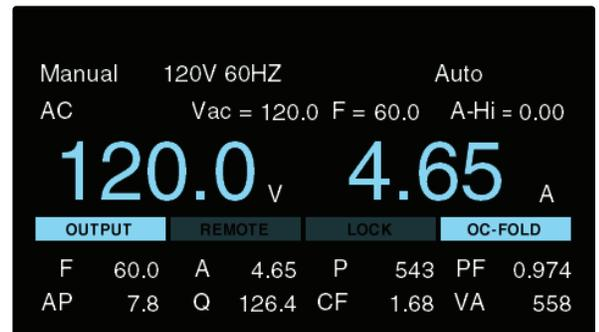
**PLC Remote** – If the PLC Remote parameter is enabled and a test is performed via a PLC remote control REMOTE will be highlighted on the screen.
