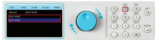
5. Use the rotary knob to highlight the file you wish to edit. Press the rotary knob to view the test parameters. Once the file name is highlighted, the user can also press the number 2 key, or the ENTER key, on the keypad to view the test parameters:
