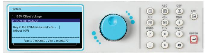
Input the Vdc measurement of the DVM.
