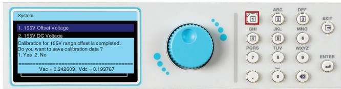
Use the rotary knob to highlight the 155V DC Voltage selection. Press the ENTER key to view the next page.
