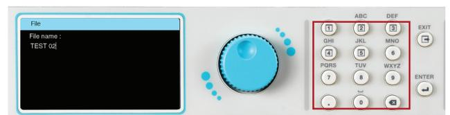
7. After entering the file name, press the ENTER key on the keypad to save the file name and display the test parameters for editing:
