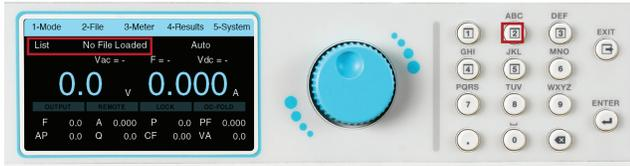
2. Once the mode has been set to List press any key to drop down the menu bar and press the number 2 key on the keypad to enter the File menu:
