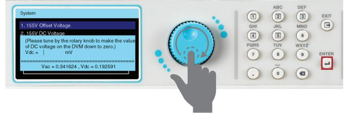
The measured value Vdc is already close to zero and this screen will be displayed. Press the 1 key to save the correction value.
