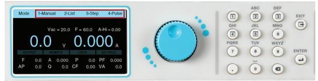
3. Using the keypad, select the desired Mode. For example, if the number 1 key is pressed the Manual Mode will be selected and the screen will display the mode and the file name that was last used in this mode.
