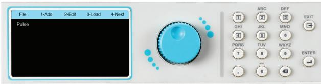
4. To start adding a test file press the number 1 key on the keypad to select Add:
