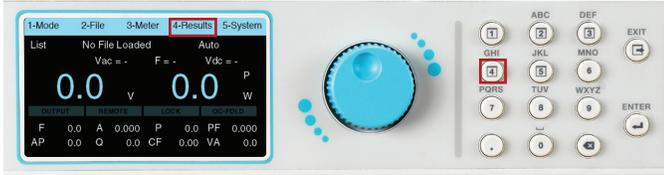
2. The Results screen will appear and the rotary knob can be used to view the results:
