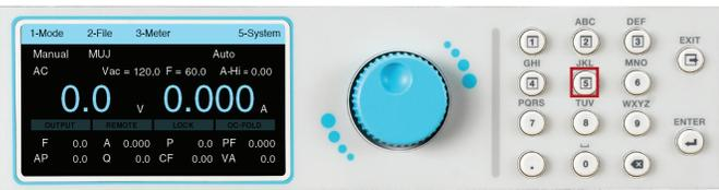
2. The System Parameter screen will open and display all the parameters available for editing. Use the rotary knob to scroll through the system parameters.
