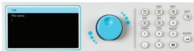
6. Use the keypad to enter a name for the test file (23 character limit):
