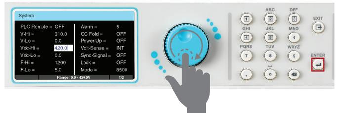
5. Rotate the knob or use the keypad to change the parameter to the desired value:
