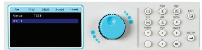
5. Press the number 4 key on the keypad to view the next page of the File menu. The next page will display the selections to Copy or Delete an existing test file. Selecting Next (by pressing the number 3 key on the keypad) will display the previous page of the File menu:
