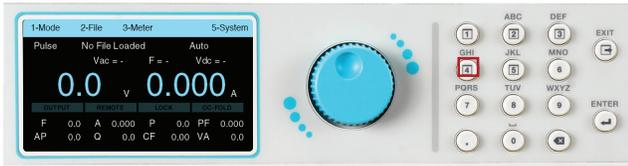
2. Once the Mode has been set to Pulse, press any key to drop down the menu bar and press the number 2 key on the keypad to enter the File menu:
