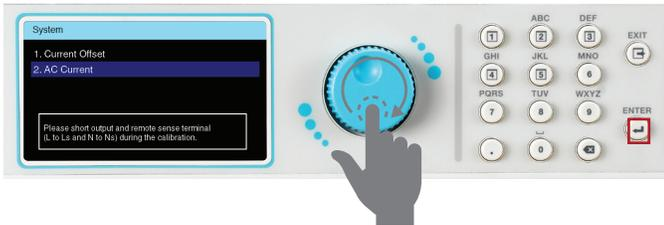
Confirm that there is a connection to the load. Press the 1 key to confirm. Reference the following table for proper resistive load values for each of the four different APT 8500 models:
