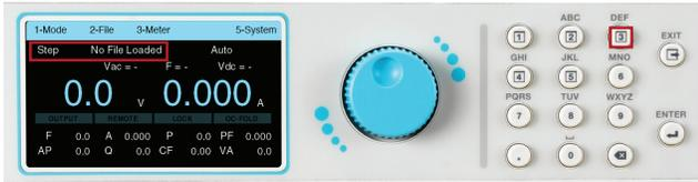
2. Once the Mode has been set to Step press any key to drop down the menu bar and press the number 2 key on the keypad to enter the File menu:
