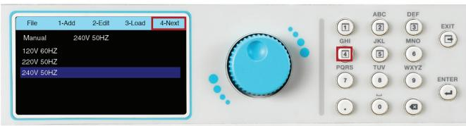
2. Use the rotary knob to select the file to be deleted. The Delete selection will appear on the menu bar, press the number 2 key on the keypad to delete the highlighted file:
