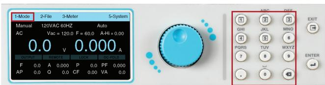
2. Press the number 1 key on the keypad to enter the Mode menu. The four selections for Mode will be displayed on the menu bar, all associated with a number.
