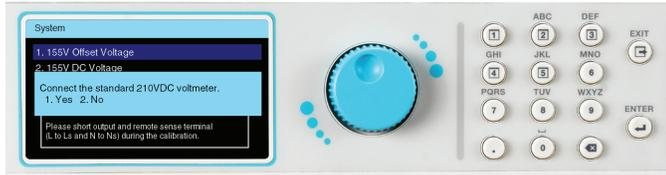
Observe the voltage measurement on the DVM, then input the “negation value” of the measurement (e.g. DVM Vdc= 1234mV, input the value “-1234” , press the . key to enter the +/- symbol).
