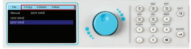
3. To copy a file, use the rotary knob to highlight the file to be copied and press the number 1 key on the keypad:
