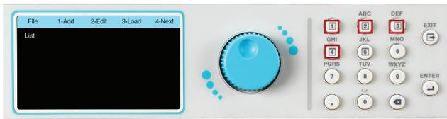
4. To start adding a test file press the number 1 key on the keypad to select Add:
