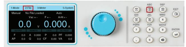
3. The File screen will be displayed and the selections on the menu bar will change. If there are no previously saved test files for Manual Mode the screen of the File menu will display the selections to Add, Edit or Load a test file on the menu bar. The Next selection on the menu bar will not do anything:
