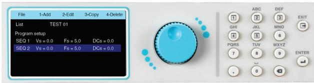
4. Once all the Program Setup parameters have been programmed and all the sequences have been created press the EXIT key on the keypad and the screen will display your newly created test file (along with other test files that may have already been saved):
