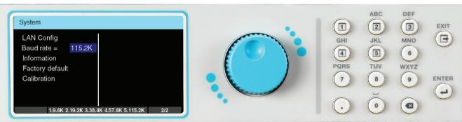
4. To edit system parameters use the rotary knob to highlight the desired parameter, press the rotary knob or the ENTER key and the parameter field will turn white with a blinking cursor:
