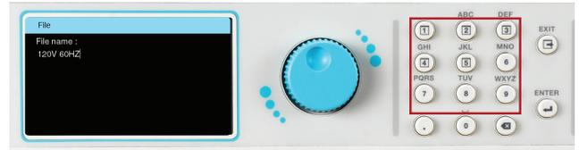
9. After entering the file name press the ENTER key on the keypad to save the file name and display the test parameters for editing:
