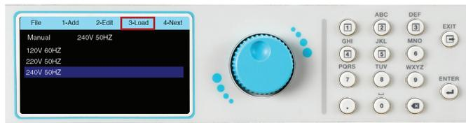
2. Press the number 3 key on the keypad to select Load and the screen will change to the test screen. The test file name that was loaded will appear on the screen:
