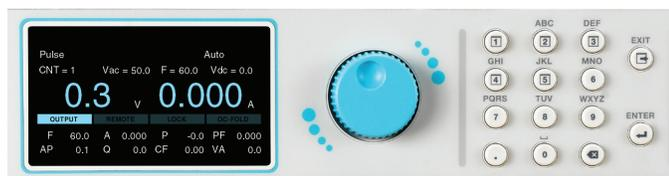
2. The user can press the OUTPUT/RESET key at any time during the test to end/abort the test.
