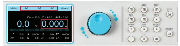
3. Use the keypad to select the desired meter to be displayed as the main meter along with voltage.
