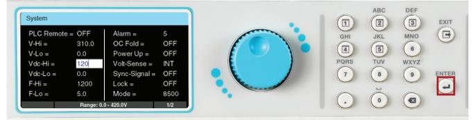
7. Repeat this process until all system parameters have been programmed as desired. Press the EXIT key on the keypad at anytime to exit out of the System menu and back to the test screen.
