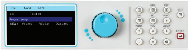
8. Use the rotary knob to highlight Program Setup or the first sequence parameters. To edit the parameters you can do one of the following: press the rotary knob, press the ENTER key or the number 2 key on the keypad. The Program Setup screen displays the following parameters:
