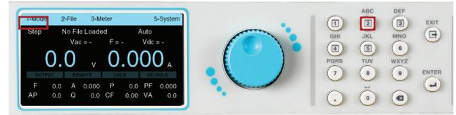
3. The File screen will be displayed and the selections on the menu bar will change. If there are no previously saved test files for Step Mode the screen of the File menu will display the selections to Add, Edit or Load a test file on the menu bar. The Next selection on the menu bar will not do anything:
