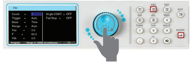
9. The sequence setup has two screens, one for test parameters and another that allows you to program additional metering. To view the sequence test parameters highlight the first sequence and press the rotary knob or the ENTER key:
