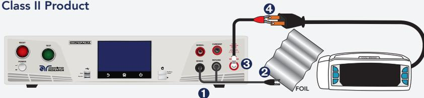
**Did you know?** If necessary, a 10 x 20 cm piece of foil can be attached to the enclosure to simulate a full hand contact to the DUT. This foil acts as the return point. The Return and Sense (-) terminal are attached to the foil. Always check to make sure you made a good connection between the DUT and the return clip.
