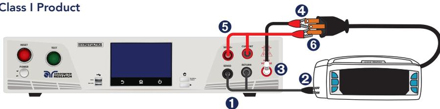
If there is no ground circuit present on the DUT, you can use test leads to connect the HypotULTRA® to the DUT.
