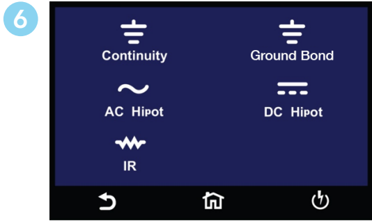
FailCHEK® Menu - Check the instrument's failure detectors.
