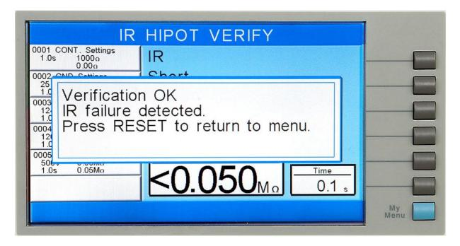
If the instrument fails the Verification (test pass, indicating the fail detectors are not working properly) the TEST button will illuminate and the following pop-up message will appear over the metering screen:
