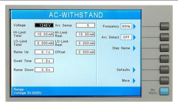
From the AC Withstand Parameter Setting screen the following parameters may be controlled: Voltage, HI-Limit Total, LO-Limit Total, Ramp Up, Dwell Time, Ramp Down, Arc Sense, HI-Limit Real, LO-Limit Real, Offset, Frequency, Arc Detect (ON/OFF), Step Name, Scanner Channel, Defaults and More. Pressing the More soft key will display the additional parameters Continuity selection (DC continuity or OFF) and Select Meter.
