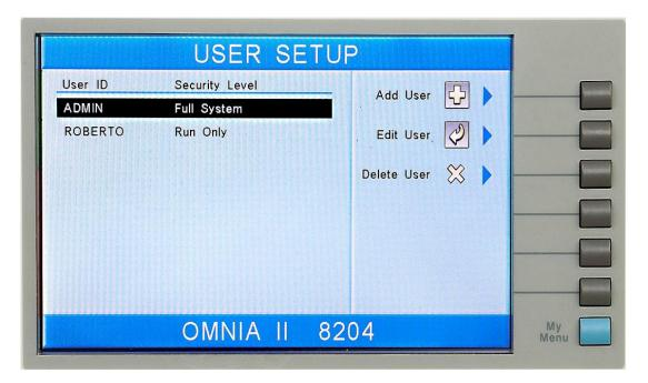
From the User Setup screen, you can view the list of users currently setup and the associated security level. The OMNIA will have a default User ID named ADMIN with Full System Access security level. This User ID cannot be deleted.
