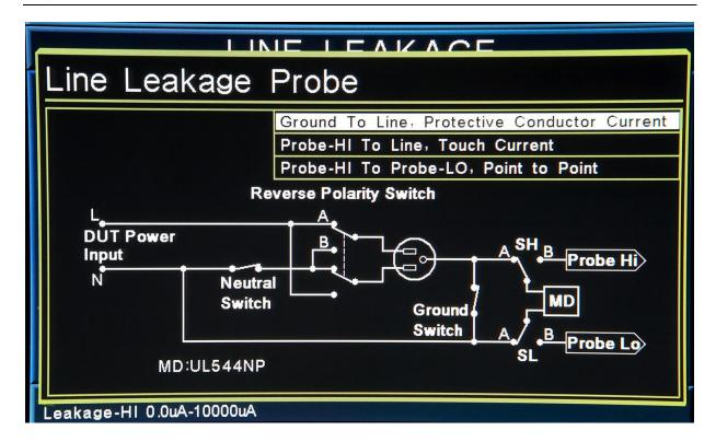
Ground-to-Line indicates the MD is connected to measure the leakage current in the line cord from the earth ground conductor back to the system neutral. This is referred to as an PROTECTIVE CONDUCTOR CURRENT TEST.
