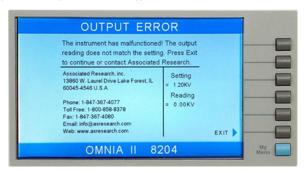
The RESET button is not active in this situation. Only the Exit soft key will allow you to return to the Perform Test screen.
