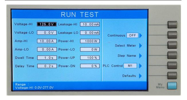
When the Power Tracking and Continuous Output options are installed, the DUT will be connected to the power source during and between test steps. If the power reading increases above the Power-UP percentage or drops below the Power-DN percentage from the previous step, then the next step will begin.
