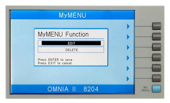
Use the up or down arrow keys to select the preferred function. The My Menu setting options are EDIT and DELETE. EDIT will allow the user to select a system, test or file
