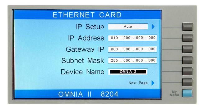
From the Ethernet Card Parameters screen, six different parameters may be accessed: IP Setup, IP Address, Gateway IP, Subnet Mask, Device ID, and Next Page.
