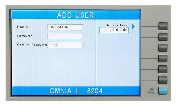
From this screen, a new user can be added by entering an alpha/numeric User ID, Password, Password Confirmation and desired security level.
