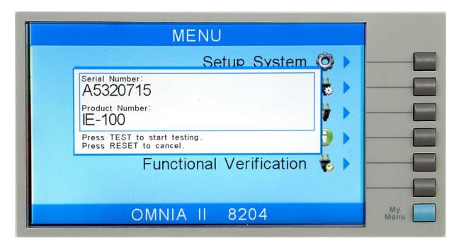
After the barcodes are scanned, press TEST to initiate the test sequence. Pressing RESET will abort the TEST sequence.
