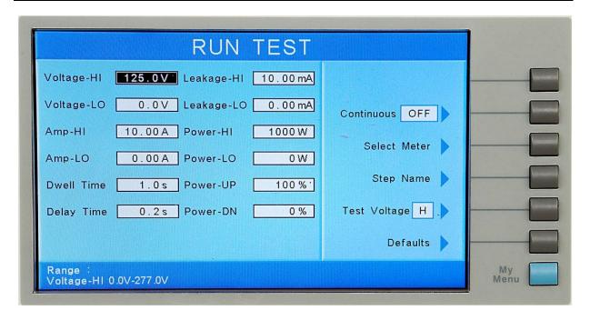
Setting the Test Voltage selection to N, L, and H will create different digital states at Bit 0 and Bit 1 of the PLC Remote Signal Output (refer to the PLC Signal Output drawing below). The different states are described in the truth table below. The "Not used" state is undefined and cannot be programmed for use.
