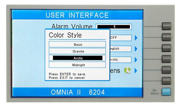
Use the up or down arrow keys to select the preferred color style setting for the unit. The color style setting options are Basic, Granite, Arctic and Midnight.
