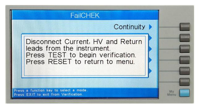
Follow the instructions given in the pop-up message and then press TEST to begin the verification process. During the Verification process the metering screen for the related process will be displayed, refer to section **5.4. Perform Tests Metering** for
