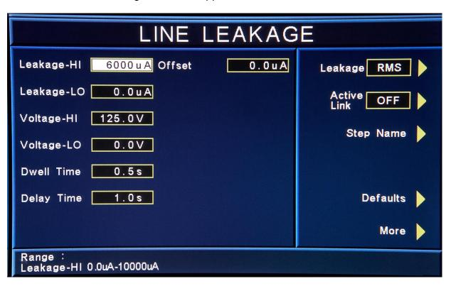
From the Leakage Current Parameter setting screen, the following parameters may be controlled: Leakage-HI, Leakage-LO, Voltage-HI, Voltage-LO, Dwell Time, Delay Time, Offset, Leakage, Active Link, Step Name, Scanner Channel, Defaults and More. Pressing the More key will bring up additional parameters: Reverse, Neutral, Ground, Measuring Device and Probe. Pressing the More soft key again will bring up additional parameters: AC Source, AC/DC, Select Meter, and Ranging Mode.
