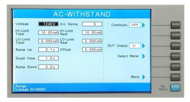
This provides additional settings to control the DUT Output L and N terminals during ACW, DCW and IR tests. When this option is installed and the DUT-HV setting is enabled in the Setup System screen an additional parameter will be available in the ACW, DCW and IR Test Parameter Settings screen. The operator can configure the DUT Output L and N terminals to O (off), H (which places them at high potential) or L (which places them at return potential). Refer to the table below for more details.
