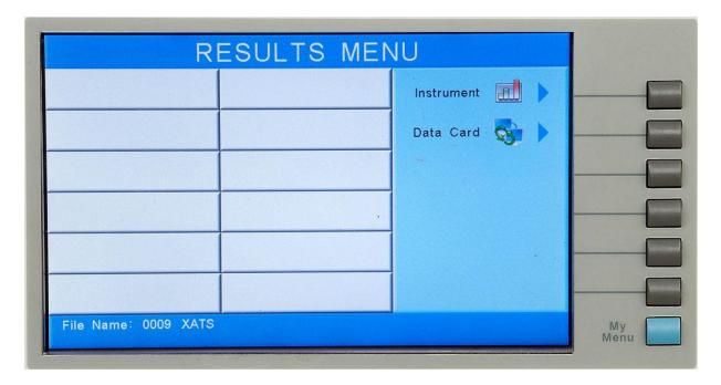
Pressing the soft key labeled Instrument will display the detailed results from the previously executed test file. Pressing the soft key labeled Data Card will display
