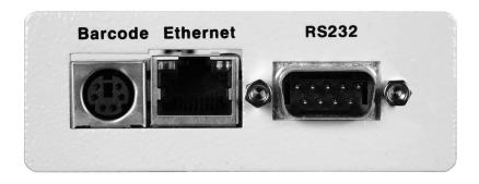
The port labeled "Barcode" is a PS/2-type connector that is used for the connection of a barcode scanner. The Ethernet port is for use with a standard CAT-5 Ethernet cable and may be connected to any compatible PC. The 9-pin D-type subminiature connecter labeled "RS232" is for connection of the OMNIA to an RS-232 communication bus.
