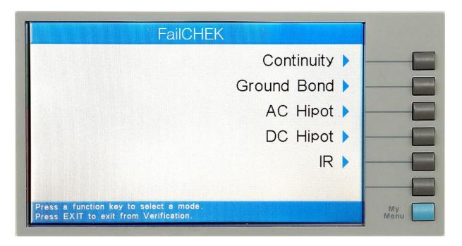
The FailCHEK Menu screen will now be displayed. From the FailCHEK Menu screen, five different Verification processes may be accessed: Continuity, Ground Bond, AC Hipot, DC Hipot, and IR.
