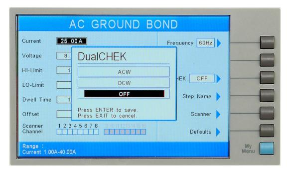
Use the up or down arrow keys to select the DualCHEK setting for this test. The DualCHECK setting options are ACW, DCW or OFF.
