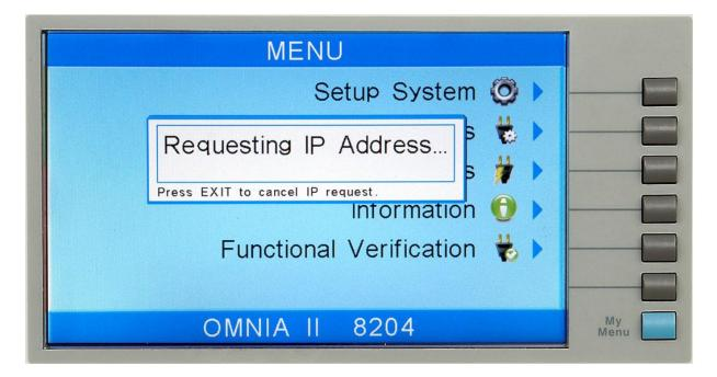
NOTE: The "Requesting IP Address..." pop-up message only appears at power up when the Ethernet Card has its IP Setup configured to AUTO.
