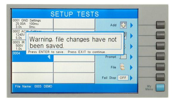
Pressing the ENTER key will store the file with the file name you gave it and go to the Perform Test screen. You may now perform a test (refer to section **5.2. Perform Tests Menu**).
