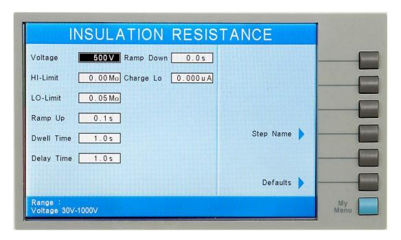
From the Insulation Resistance Parameter Setting screen the following parameters may be controlled: Voltage, HI-Limit, LO-Limit, Ramp Up, Dwell Time, Delay Time, Ramp Down, Charge-LO, Scanner Channel, Select Name and Defaults.
