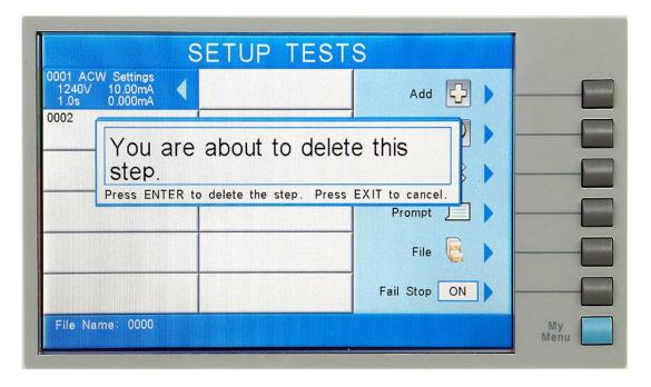
Press ENTER to confirm and delete the selected step or EXIT to cancel and return to the Setup Tests screen.
