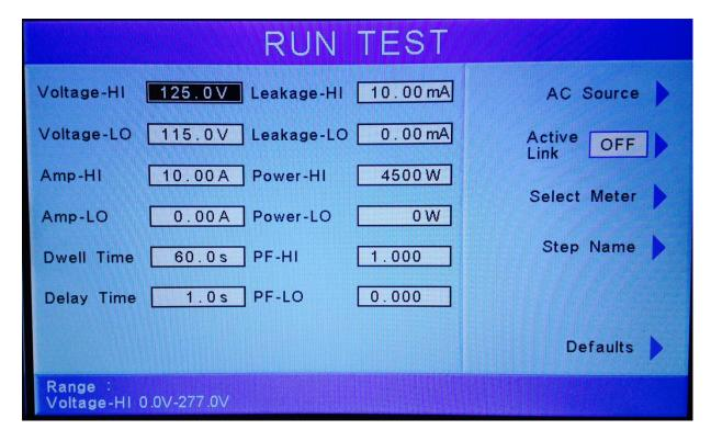
From the Run Test Parameter Setting screen, the following parameters may be controlled: Voltage-HI, Voltage-LO, Amp-HI, Amp-LO, Dwell Time, Delay Time, Leakage-HI, Leakage-LO, Power-HI, Power-LO, PF-HI and PF-LO, AC Source, Active Link, Select Meter and Step Name.
