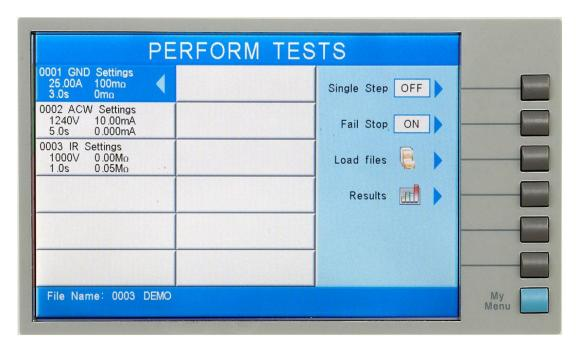
The Perform Tests screen is the main operational screen of instrument. From this screen individual steps are monitored while the test is being performed. At the end of a sequence of tests, all of the step results may be recalled via the "Results" soft key on this screen. This screen may also be used to debug test files with the use of the single step and fail stop functions.
