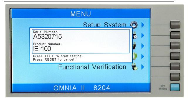
After the barcodes are scanned, pressing TEST will initiate the test sequence. Pressing RESET will abort the TEST sequence.
