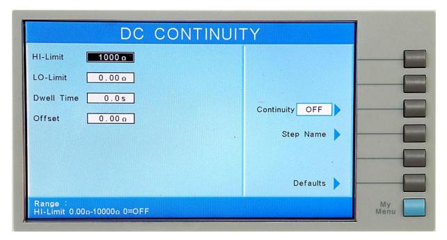
The "Continuity" selection is short for continuity connection and refers to which connection points may be utilized for the continuity measurement. The new continuity parameter has three toggle selections MAINS, GND, and OFF.
