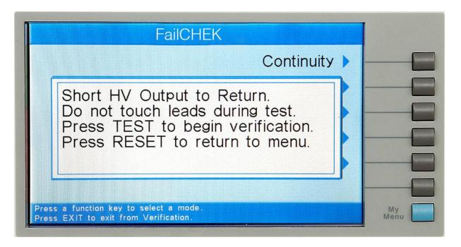
Follow the instructions given in the pop-up message and then press TEST to begin the verification process. During the Verification process the metering screen for the related process will be displayed, refer to section **5.4. Perform Tests Metering** for more information.
