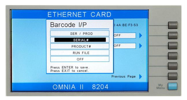
The Barcode I/P parameter can be set to SERIAL#, PRODUCT#, SER/PROD, OFF or RUN FILE. When the setting is SERIAL#, PRODUCT# or SER/PROD, the user can scan barcodes in the Perform Tests screen before the test is started. When a barcode is scanned, one of the following messages will appear on the display.
