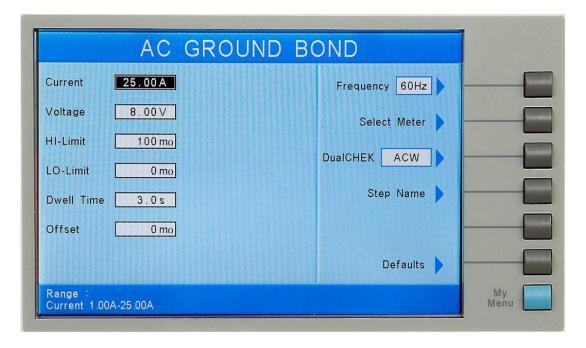
From the Ground Bond Parameter Setting screen, the following parameters may be controlled: Current, Voltage, HI-Limit, LO-Limit, Dwell Time, Offset, Scanner Channel, Frequency, DualCHEK, Step Name and Defaults.
