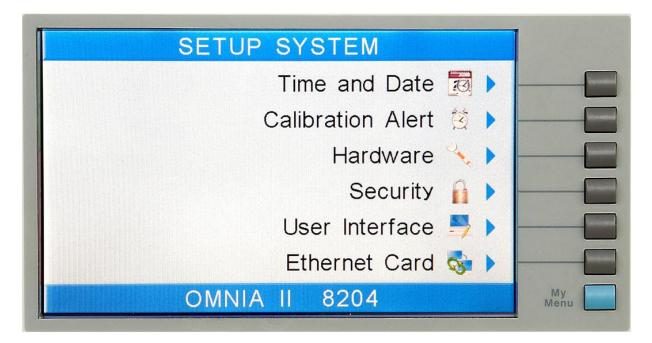
To access the Ethernet Card Menu, press the "Ethernet Card" soft key from the Setup
