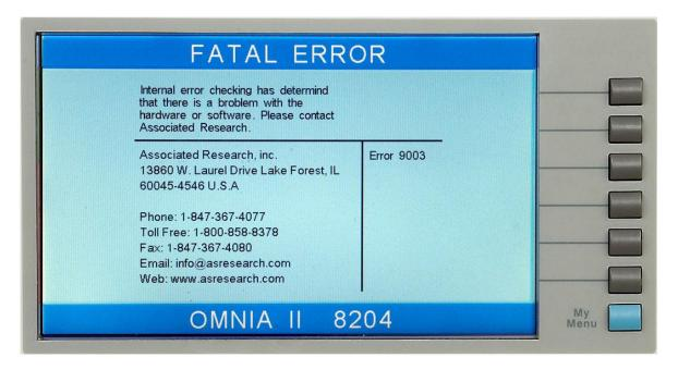
This type of failure permanently locks the instrument in the "Fatal Error" mode and requires that the instrument be serviced by Associated Research. The following Fatal Error identification numbers will represent the type of failure that has occurred:
