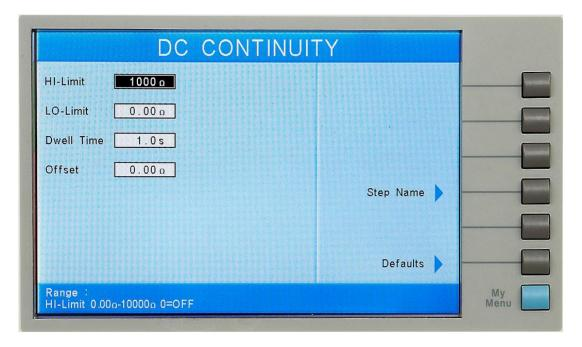
From the Continuity Parameter Setting screen, the following parameters may be controlled: HI-Limit, LO-Limit, Dwell Time, Offset, Scanner Channel, Step Name and Defaults.
