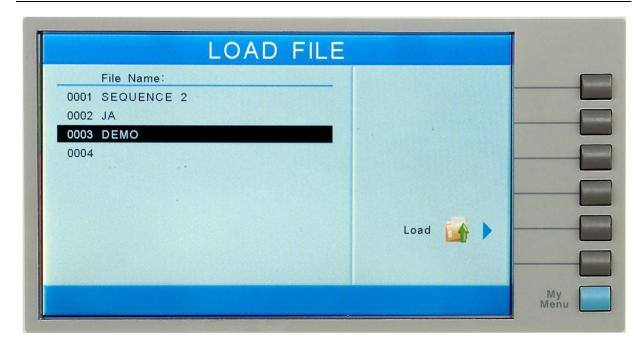
Using the up and down arrow keys, scroll the highlighted area to the File you would like to load and press the "Load" soft key. The file you selected will now load and the screen will revert to the Perform Tests screen.
