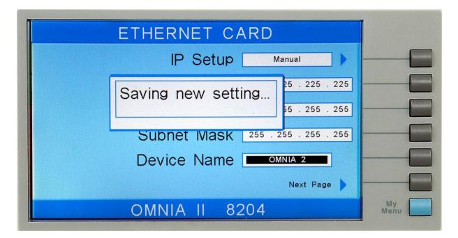
The Ethernet Card will attempt to re-establish a connection with the server anytime the user modifies a parameter and exits the Ethernet Card Parameters Menu or uses the command set at the end of this option description. Thus, if the IP Setup is set to AUTO, the Ethernet Card will request a new IP Address every time a parameter is edited and, as a result, the "Requesting IP Address. . ." message will appear.
