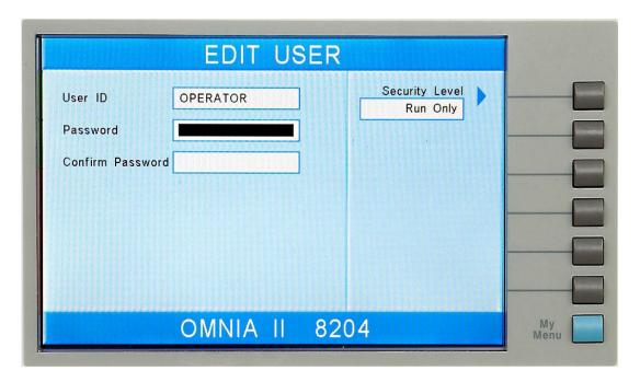
From this screen, the User ID, Password and Security Level can be changed by entering an alpha/numeric User ID, Password, Password Confirmation and desired security level. Please refer to the "User ID", "Password", "Confirm Password" and "Security Level" sections above for more information.
