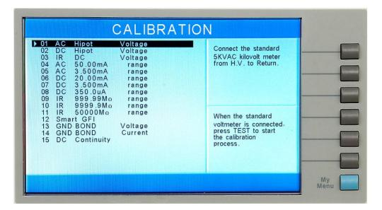
The Calibration screen is separated into three sections. The left half of the screen lists all of the calibration points necessary for an accurate calibration of the instrument. The right half of the screen is split into two smaller screens. The upper right section of the screen displays meter and load information required to perform the selected calibration. The lower right section of the screen contains prompts that will help guide you through the calibration process.
