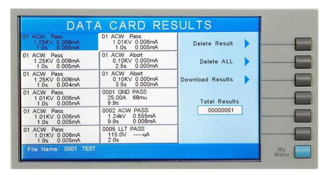
From this menu, the user can view the stored results, delete results, and transfer the results to the external USB Flash memory drive. To navigate through the results use the up, down, left and right soft keys on the OMNIA II front panel. The following message will display if the Delete Result soft key is pressed:
