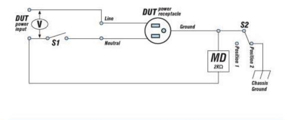
When the Leakage-HI trip limit is set to 0, S2 is placed in position 2 which disables the earth leakage test and connects the neutral of the DUT input to the ground of the DUT.
