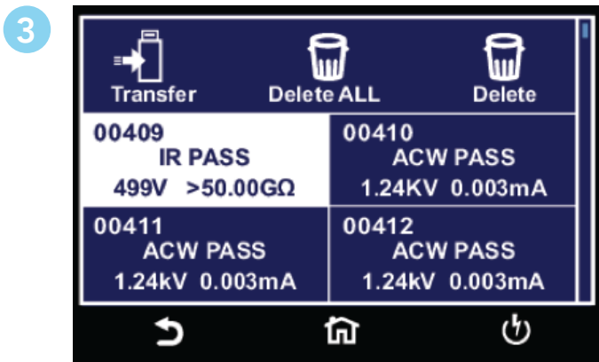
Press transfer to begin exporting internal memory results.
